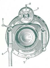
It is fitted with Iris Diaphragms which are regulated by moving the lever 5 to the right or left. The openings are in accordance with the uniform system and are indicated on the scale.
