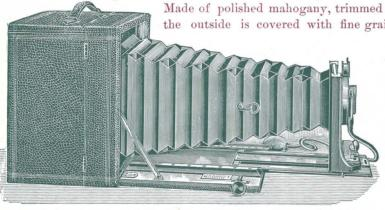
back with both vertical and horizontal swings so arranged that they are easy and convenient to use. The long draw is obtained by the double bed, one part of which slides on the other, and rack and pinion focusing movement as shown in cut. This allows the use of very long focus lenses. The  $5 \times 7$  having a draw of 21 ins., and measures when closed  $9\frac{1}{2}$  ins. long,  $9\frac{1}{4}$  ins. high and  $5\frac{3}{4}$  ins. wide, weighs but  $6\frac{1}{2}$  lbs., yet
