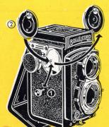
To change counter mechanism: Open back, loosen screw (1), exchange counter dial mechanism (2) and tighten screw.
