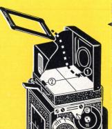
Slip ground glass mask under clip at the front (1), drop rear into place and fasten by pressing locking lever (2). Figures on mask must be legible right-side-up.
