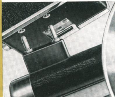
To attach flash gun to your C3, simply plug it into the side of the camera. Caution: Do not have a flash bulb in the gun when attaching it to the camera.
