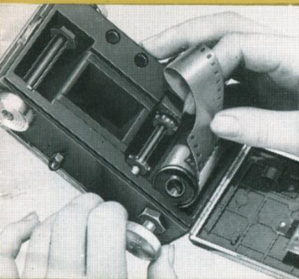
Pull out Rewind Knob on the bottom of the camera, and insert the 35mm cartridge. Then push in Rewind Knob (it may be necessary to turn it slightly).
