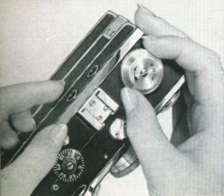
Turn Winding Knob as far as it will go without forcing. Hold down Film Catch, and turn Winding Knob about a quarter of a turn. Release Film Catch and wind as far as knob will turn. Repeat this operation again in order to take up proper amount of film leader.
