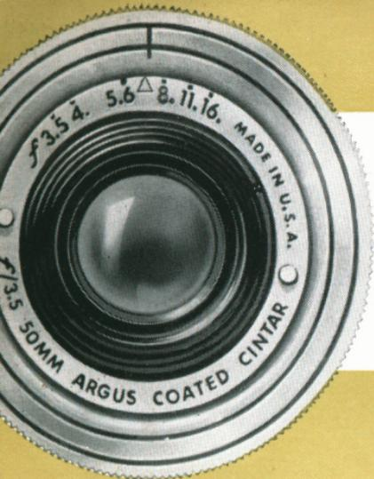
Smallest opening is provided at f:16. Turning dial clockwise to next f-stop number opens lens for twice as much exposure as at each previous setting (except f:3.5, which adds only half again as much as at f:4). Turning dial in opposite direction cuts exposure in half at each f-stop.
