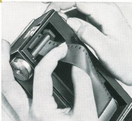
Thread end of film completely through the slot on the Take-up Spindle. Turn Wind Knob approximately one-half turn until film folds under itself and is secure on shaft.
