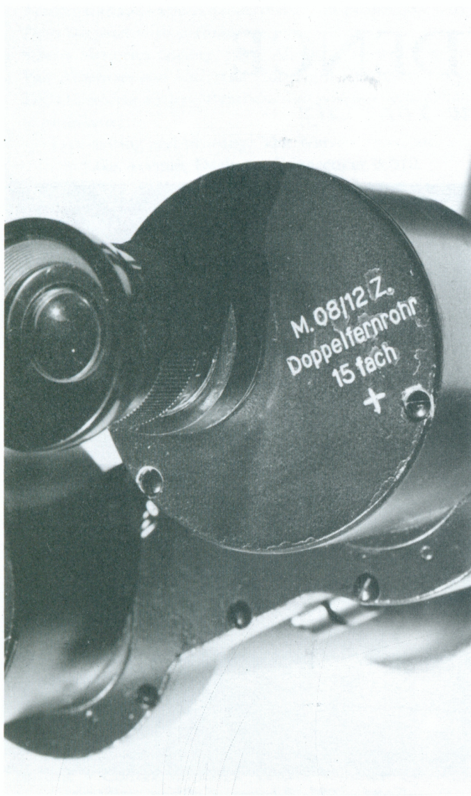
15x60 binocular with the Zeiss/Wien (Zeiss/Vienna) trademark is marked with a white "+", dates from around 1925.
