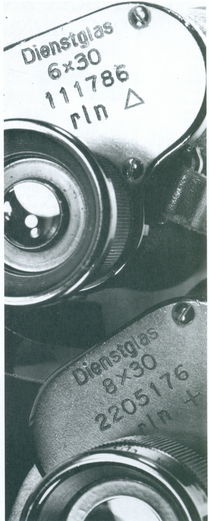
6x30 Zeiss Jena binocular (top) carries a triangle mark; 8x30 instrument carries "+" mark.
