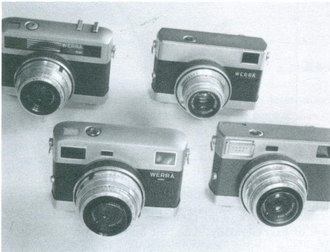
A quartet of Werras. Top row, left to right: Werramat (version 4), Werra I (version 2). Bottom row, left to right, Werramatic (version 3) and Werra IV (version 1).
