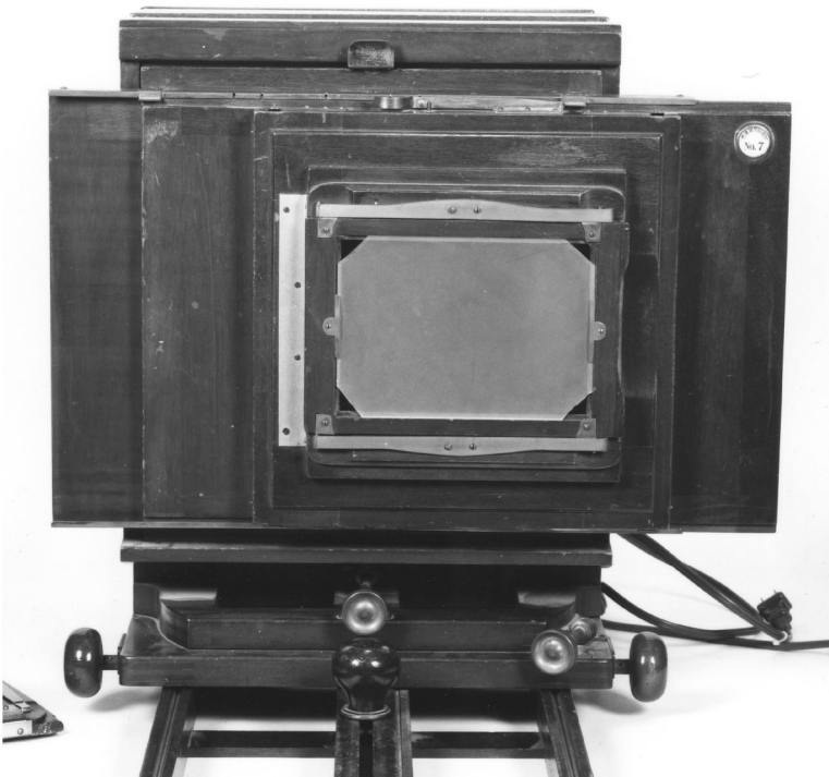
No. 7 5x7 back shifted to utilize the split back feature that allows two 3½- x 5-inch exposures on one sheet of film.
