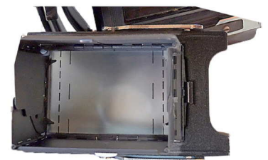
Figure 6 An alternate ground glass was found that had various image formats marked on the glass.
