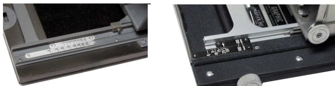
Left to right; Vernier and modified Vernier scales. Scales are numbered to correspond to different lenses.
