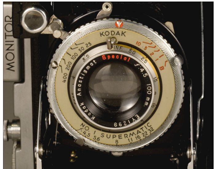
Kodak Anastigmat Special (c.1940) lens in a No. 1 Supermatic shutter on a Kodak Monitor Six-20 camera. Image courtesy Todd Gustavson, Technology Curator, George Eastman House.
