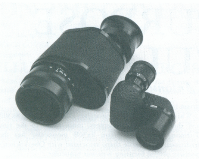
Porro prism version of the 8x30B dwarfs its smaller relative, a postwar 8x21 Turmon.
