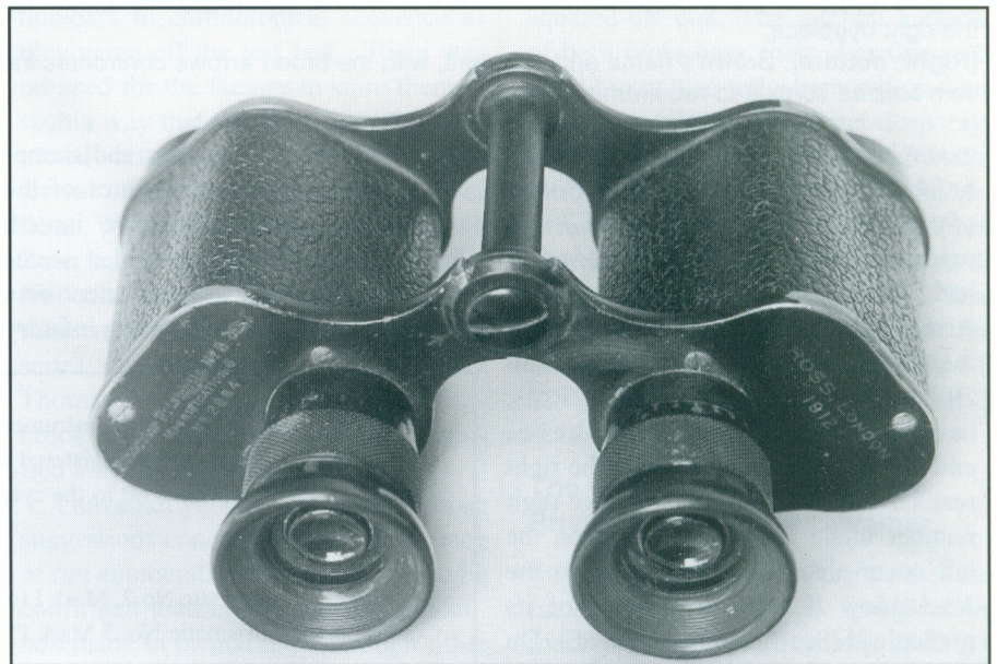
Binocular, Prismatic, No. 3 Mk I , dated 1912, produced at the Clapham works. This binocular shows the characteristic Ross design, where extensions to the cover plates form the hinged arms of the upper and lower bridges. WR/K435.
