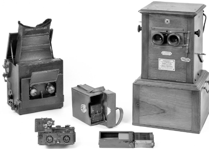
Left to right: Stereo Auto Graflex, Richard Verascope with early roll film back and accessory self-timer, case for glass plate magazine showing operation of plate changing mechanism, and Taxiphote slide viewer.
