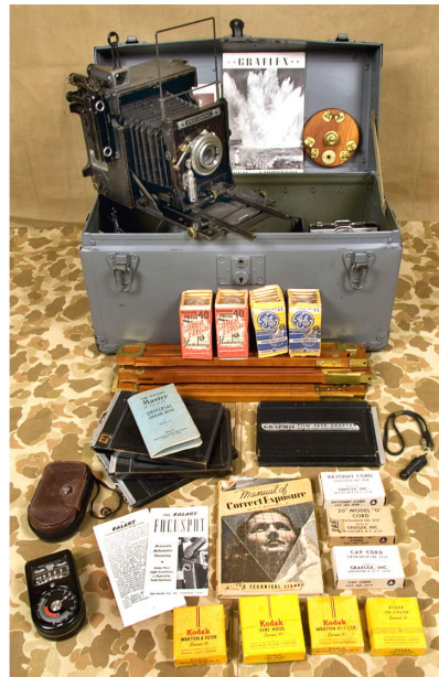
Figure 4. Contents of the Speed Graphic U.S. Navy Anniversay 4x5 camera set: Here is a typical assortment of accessories and components that make up this kit. The camera itself is supported by a Folmer Graflex wood tripod and head (here disassembled). There are Wabash and GE-brand flashbulbs, 12-exposure film pack adapters, a few double-sided film holders for 2 exposures, Weston Master Model 715 Universal Exposure Meter, various manuals concerning the Focuspot rangefinder and the
