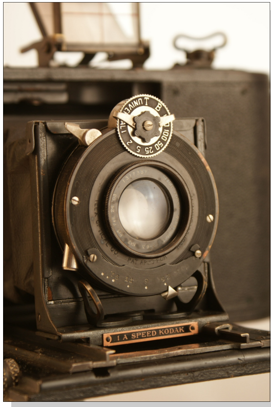
Speed Kodak, serial number 1993, fitted with a Zeiss Kodak Anastigmat F/6.3 No. 2 lens (focal length of 5") in an Ilex Optical Co. leaf shutter.
