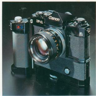
Canon makes a total of two motor drives for the F-1, both of which use Canon's two-motor system: one motor for film advance and one for shutter release. The Motor Drive MF is easily attachable to an F-1 camera with no modification necessary. Just remove the camera's bottom cover and screw the
