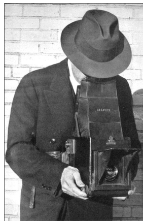
"The Graflex ready for action. The position shown is the most effective way of holding and operating this camera."
