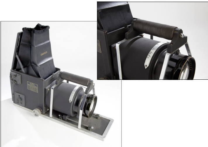
Jim Chasse's 4x5 R.B. Series D, with Zeiss Jena 400mm f/4.5 lens.
