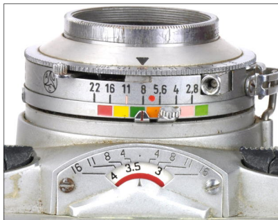
Figure 10 Universal Spectramatic band aperture adjustment and distance scale. Photo by John Wade.
