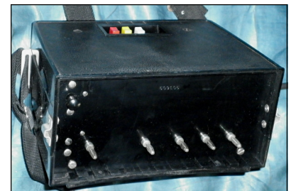
Picture 4. High voltage top half, with safety discharge switch at top left.
