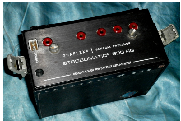
Picture 3. Battery pack and DC step-up lower half.
