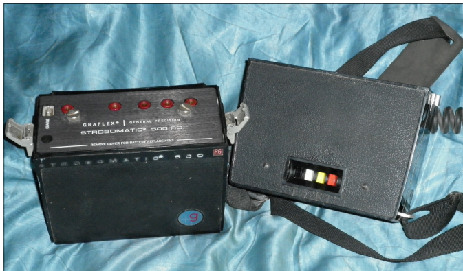
Picture 2. Battery pack (left) and capacitor unit (right).
