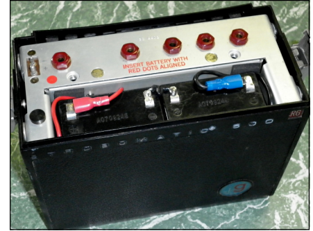
Picture 8. New batteries (12 volts). A perfect fit..
