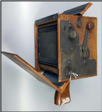
Left to right, model B prototype, prototype open, and actual production camera. It appears that film loading was simplified by removing the corner post.
