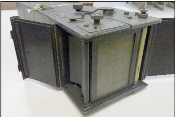
Left to right, model B prototype, prototype open, and actual production camera. It appears that film loading was simplified by removing the corner post.
