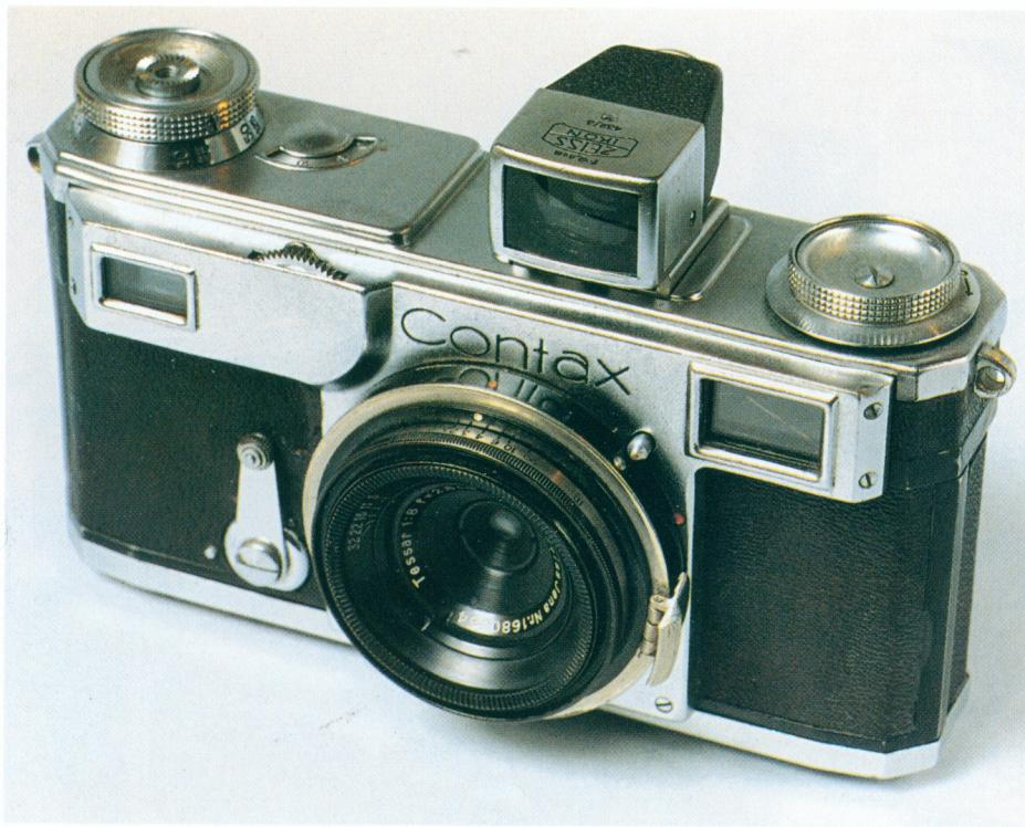
A Contax II with Tessar 2.8 cm f/8 equipped with the special viewfinder for 2.8 cm focal length, Zeiss catalogue 432/3.
