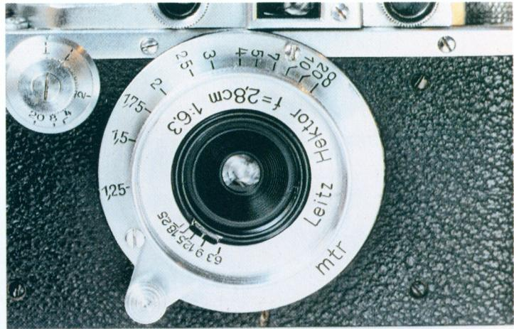
A close up of the Leitz Hektor. At the bottom left, the classic Leitz focusing "bell". The Leica's aperture control ring is also difficult to operate.
