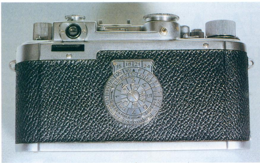
*A rear view of the Janua, with a single eyepiece for the viewfinder and coupled rangefinder, light meter and calculator.*
