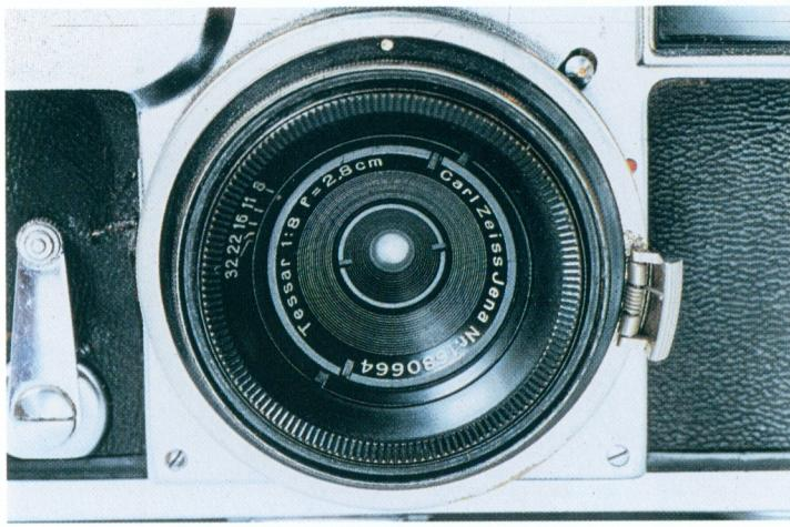
A close up of the Zeiss Tessar. Note the difficult handling of the inner aperture control ring.
