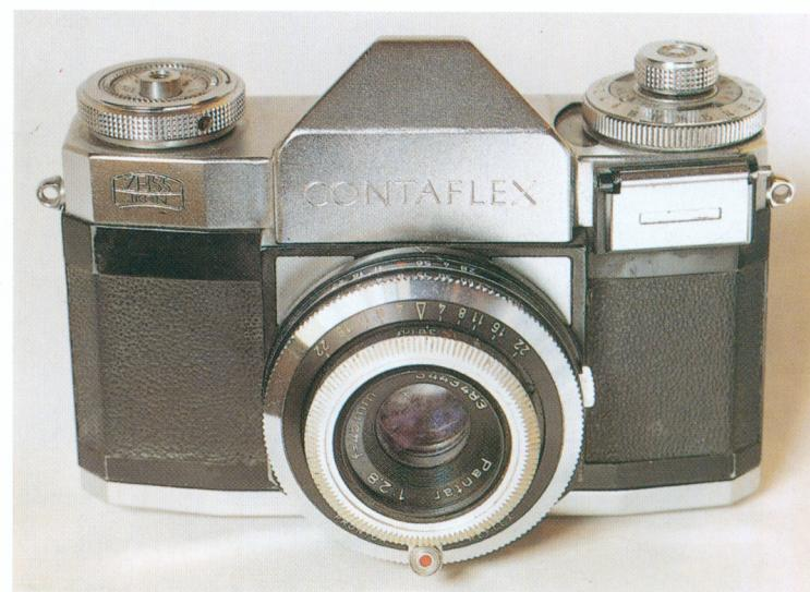
*Contaflex Beta, similar to the Contaflex II, with built in light meter and cheaper Pantar lens*
