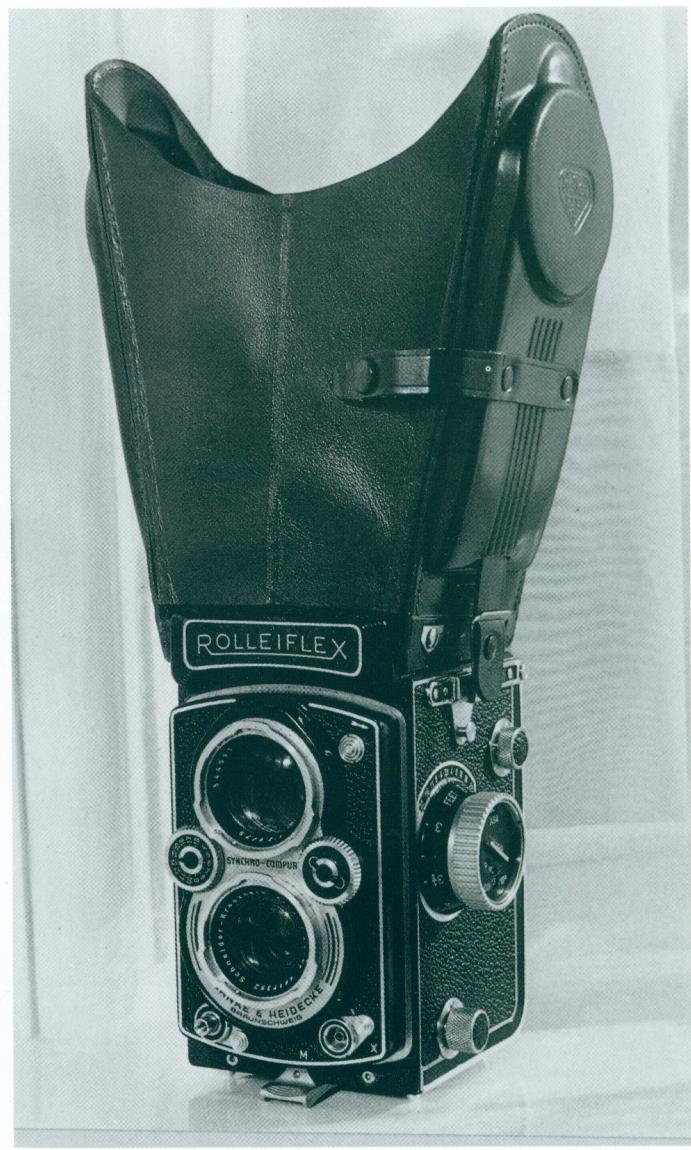
A very useful accessory for the 3.5B Rolleiflex was the Binocular Focusing Hood (PR 287). The binocular focusing hood could be folded flat when not in use and was constructed in the highest quality brown leather. It was fitted over the existing focusing hood and excluded all extraneous light from the focusing screen. Two magnifying fully adjustable lenses were fitted inside the hood.
