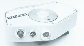
All Hycam II optical heads can be fitted with optional LED timing lights. A built-in crystal controlled timing pulse generator is also available for use with the LED timing lights. Selectable frequencies are: 100,1,000 and 5,000 Hz. A 3-position rotary switch is located on the bottom surface of the optical head to select the desired pulse rate. A 2-pin connector adjacent to the rotary switch accepts externally applied timing or event signals.
