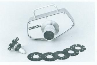
A full frame optical head with sprocket and rotating prism assembly is illustrated above. Six separate shutter discs are easily exchanged to provide shutter speeds to one microsecond. Full, ½ and ¼ frame optical heads are interchangeable between 100, 400 & 2,000 foot Hycam II cameras.
