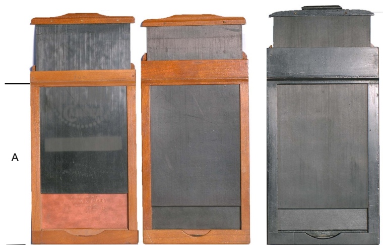
A B Premo, EKC, Graflex 1904 patent. Fiber board center. Spring plate holder. Tongue on faces.
