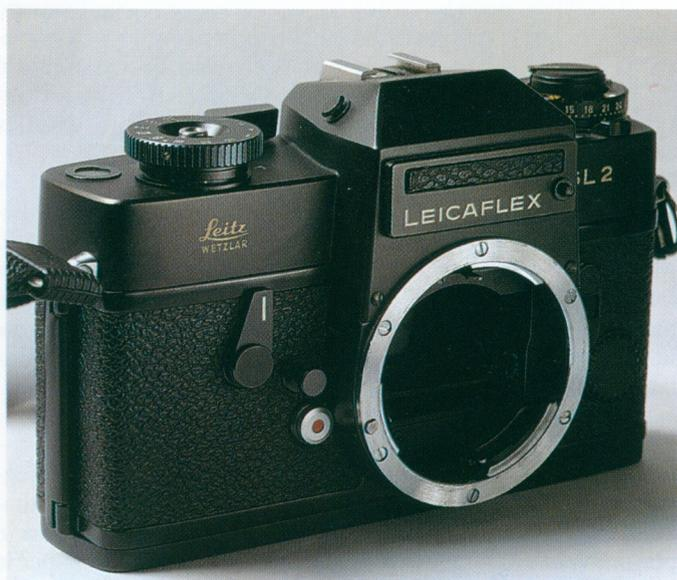
Black finish Leicaflex SL2 body with new type lens release button.
