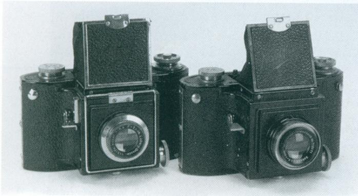
*Noviflex, Eichapel, Germany. 120-rollfilm camera, first model, with a Schneider Xenar 75mm f/3.5 lens and a Noviflex camera, 120- roll-film, second model, with a Ludwig Victor 75mm f/3.5 lens.*
