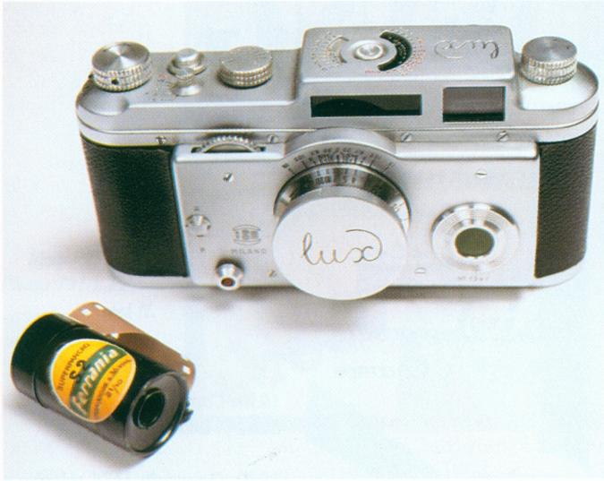
ISO LUX with original lens and cover next to an original Ferrania film cassette. Clearly evident on the camera are the viewfinder windows and the round one of the vertical rangefinder.
