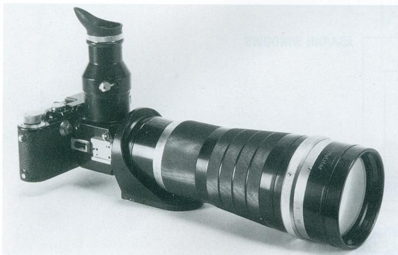
*Leica III with a PLOOT reflex housing and a Leitz Telyt 400mm f/5 lens.*
