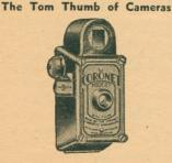
Takes 6 pictures size ½x% inches; makes perfect enlargements to 5x7 inches. Measures only 2½x1¾x1¼ inches and weighs only 1¾ ounces. Equipped with a sharp Taylor Hobson Meniscus lens with F:10 aperture; fixed focus. Instantaneous shutter (1/30th second) equipped with safety slide to eliminate accidental exposures.
