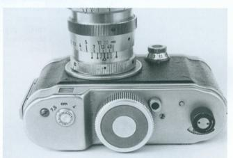
Robot II F 57186-5 series without markings indicating a specific branch of the military, including chrome top plate, no flash mount, aperture scale from 1/2s to 1/500s. On the top plate, above the finder, a knob that rotates when pressed varies the field within the viewfinder from 7.5cm to 4cm.
