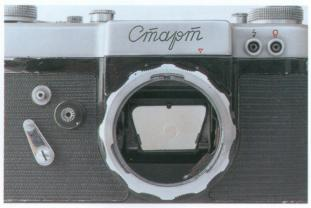
Start, detail of front with lens changing catch and breechlock mount, synch socket, self-timer lever, shutter release button and focusing wedge lowered.
