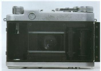
Condor II with back open. Interior with film transport mechanisms is similar to that of the Condor and is the product of the same engineering design.
