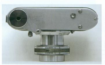
Condor II base plate. Note the fixed feet, extractable support foot, film release button and serial number.
