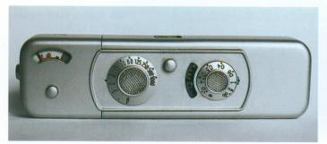
Minox BL with CdS meter - top deck with controls.
