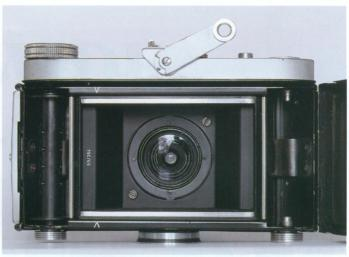
Veriwide, open, seen from behind. Note the rear lens very close to the film plane and the serial number 59/284 in which 59 could indicate the year of manufacture and 284 the camera number.
