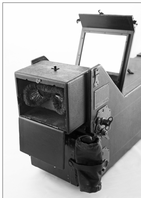
A second mirror reflects the ground glass image to the view finder when used in the horizontal position.
