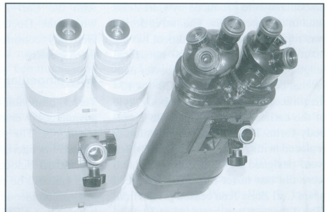
Two postwar 80/500 telescopes. The one on the left has two powers, (20× and 40×) and other, with 20×, 31× and 50× turrets, was designed for border observations. Figure 10
