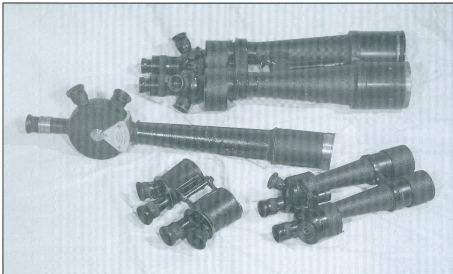
An array of early Zeiss turret instruments, including the dossefernrrohr (roof prism) telescope and the marine revolver binocular. Figure 2
