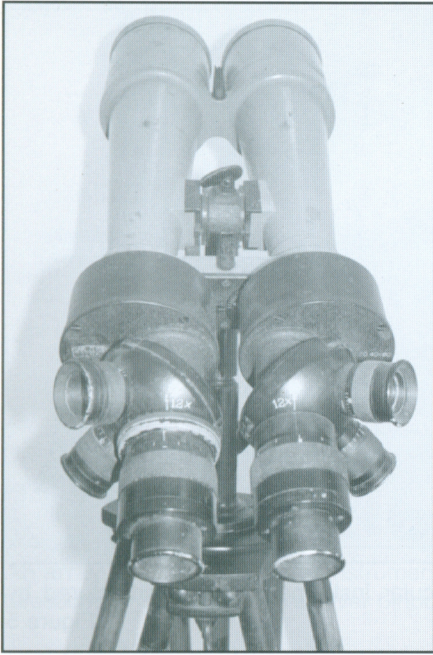
◀ An Asempi from World War I as refurbished, and the lenses coated, by Zeiss. Figure 7
