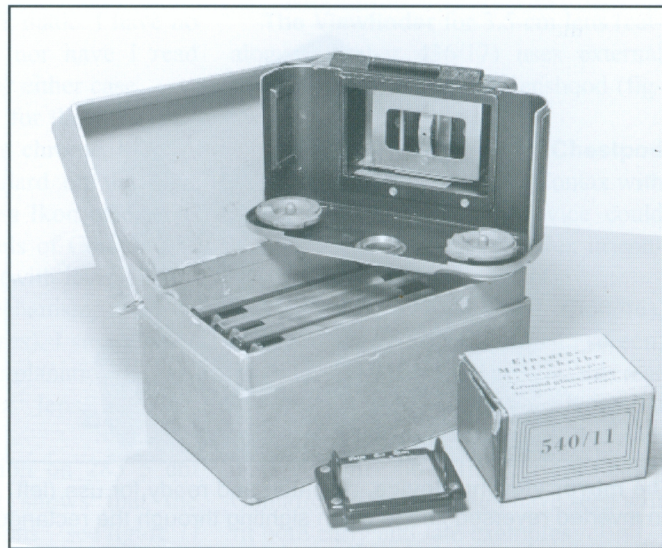
Plate back adapter (860/13) in its original box. The plate/film chassis is on the box; ground-glass adapter in front. Figure 14
