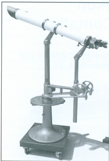
An Asal binocular telescope on its substantial stand (above left) and a closeup of its turrets (above right). Figure 14
