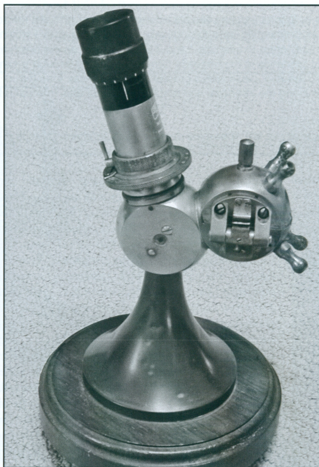
The Zeiss Butter Refractometer, developed by Pulfrich from Abbe’s original refractometer. This example was made in 1939 and sold in the US the next year; the softwood base is not original, and the thermometer is missing.
