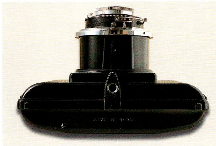
Ferrania Astor with lens extracted seen from bottom plate – the MADE IN ITALY inscription, threaded hole for the tripod and M X synch selector are visible
