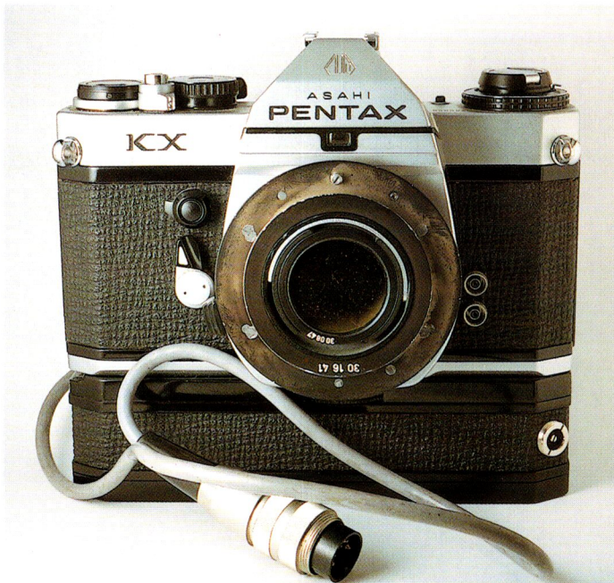
Pentax KX Motor Drive with motor, connecting cables, coupling ring and limiting cone inserted in the lens changing catch
