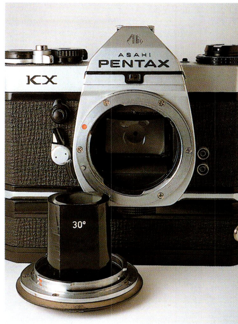
Pentax KX Motor Drive with ring and 30° cone extracted
