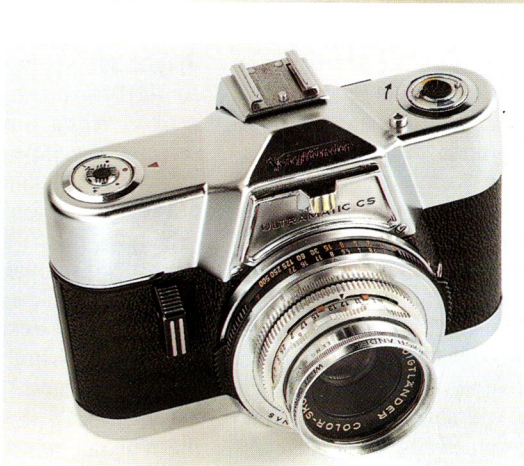
1965 Ultramatic CS with internal TTL-reading CdS exposure meter.
