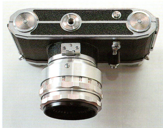
Detail of base plate with folding foot and tripod bush
