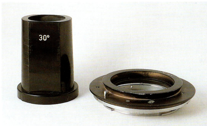
Close-up of ring and 30° image limiting cone
