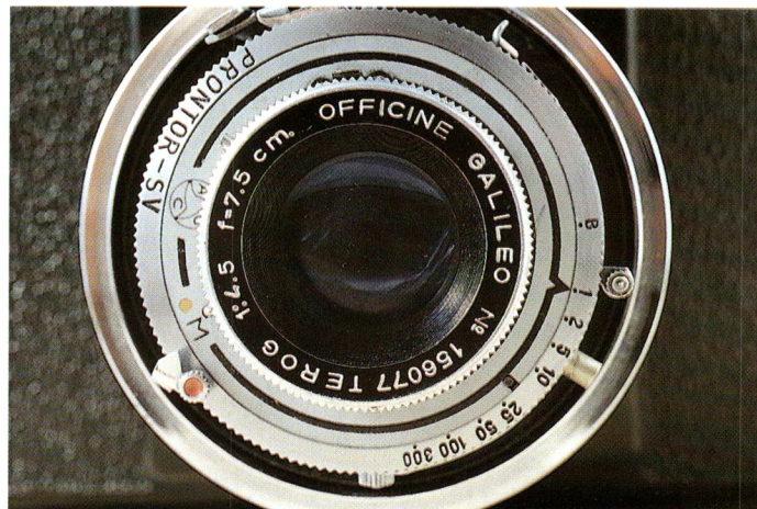
Detail of the Galileo Officine Terog 1:4.5 f=7.5cm and Prontor SV shutter
