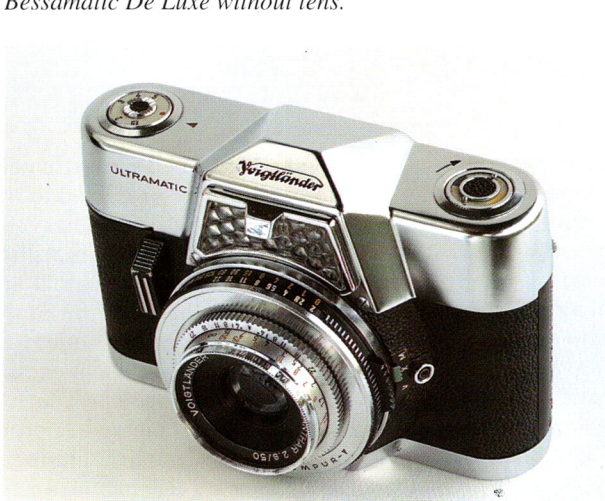
1963 Ultramatic with external selenium exposure meter.
