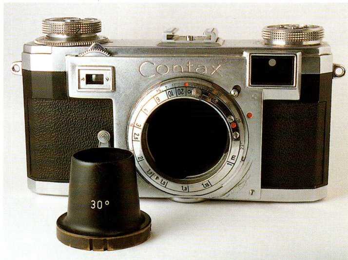
Contax IIa with limiting cone extracted
