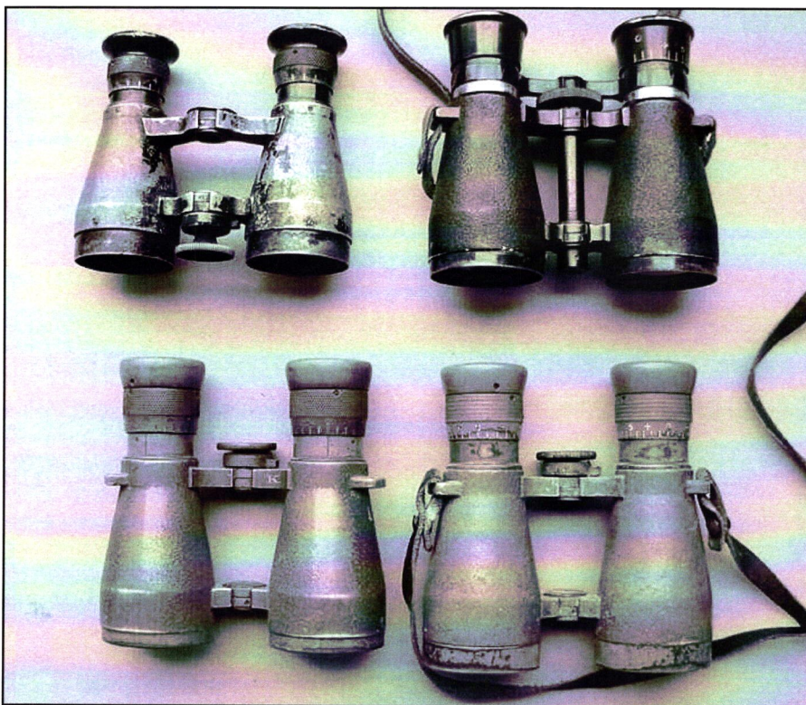
Four models of the Goerz "Fernglas 08." Top row, left to right: the 5x35 model for Switzerland, serial no.145393 (1908), and the Armeegalilei 6x, serial no.162891, also 1908. Bottom row, two Fernglas 08 — the short model 6x40, no. 10402 of 1908, serial no.157153, and the long model 6x38, no. 64045 of 1916, serial no. 407040. Figure 11
