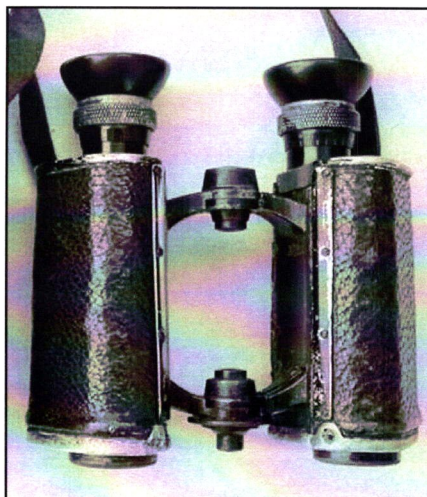
C.P. Goerz “dismantling” binocular from 1902. This 9×20 civilian version (serial no. 36621) was easily disassembled in the field for cleaning. Figure 7
