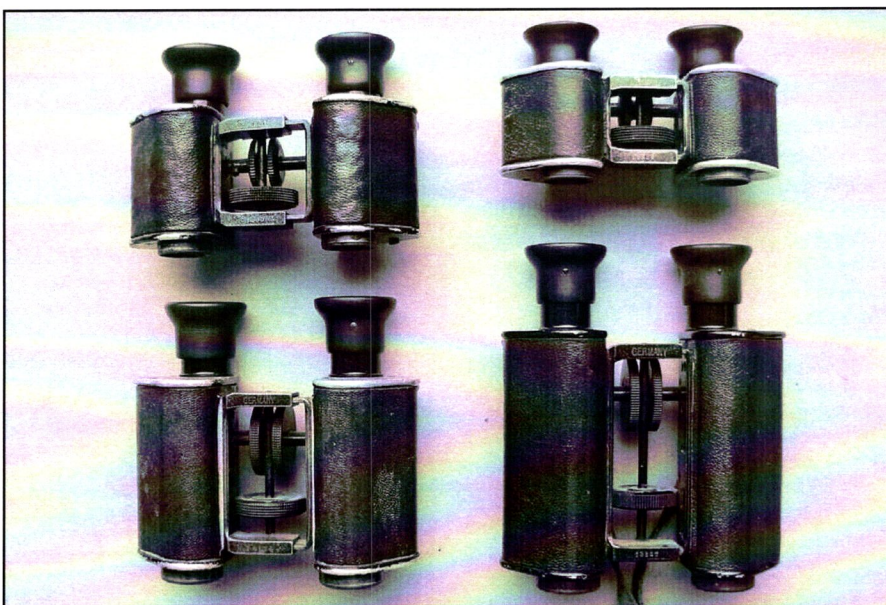
The first Goetz prism binoculars, dating from 1897. These are the 3, 6, 9 and 12-powered Trieder Binocles. Note the center-wheel focusing. Figure 5
