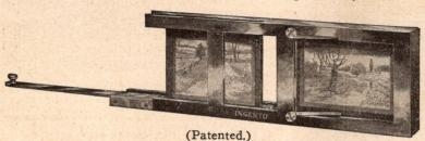
This Carrier is especially designed to secure a dissolving effect with single stereopticons. Its operation is simple and rapid. The slide is dropped into the slot at top of the Carrier and pushed into place by means of the lever. When the next slide is to be inserted, while the former slide is still projected on the screen, the same operation of the lever carries the
