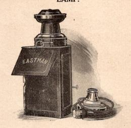
A strong, sturdy and sensibly constructed dark room lamp, mechanically correct as to ventilation, and simple to clean. The front glasses fit into light tight grooves, the ruby glass being double thickness and fitted into a metal frame with lifting ring, the orange glass, also removable, fits in a groove in front of the ruby glass.
