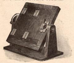
The Swivel Printing Frame is a new device for use in printing Velox or other Gas Light Papers. In large printing departments this apparatus will save its cost many times over, as it enables four operators to print at one light, without the loss of time.
