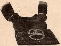
For loading plate holders and for changing plates into Ingento Developing Tanks in daylight. The plate holders and a box of plates or developing tank are put into the bag at one end. The bag is then closed with glove fasteners. The hands are inserted through the sleeves (which have rubber wrist bands) and the plates are then easily changed without loss of time.
