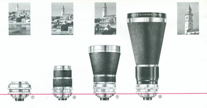
① SKOPAREX f 3.4/35 mm wide-angle lens of six elements and with 63° angle of view. ② Special SKOPAGON f 2/40 mm lens of nine elements and with 58° angle of view. ③ COLOR-LANTHAR f 2.8/50 mm standard lens of three components and with 48° angle of view. ④ COLOR-SKOPAR f 2.8/50 mm standard lens of four elements and with 48° angle of view. ⑤ SEPTON f 2/50 mm standard lens of seven elements and with 48° angle of view.
