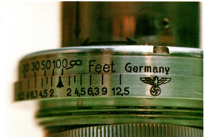
Kriegsmarine Summar lens with the inscriptions "Germany" and "Reichsadler" and distances given in feet, on a lens designated for export.
