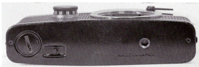
Base of Olympus Pen FT with battery housing.
