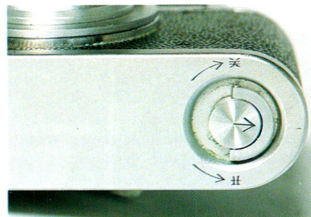
Detail of base opening key with the words "open" (kai) and "close" (guan) written in Chinese.
