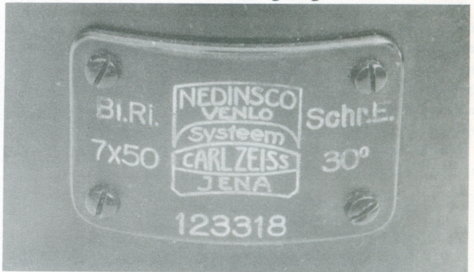
Closeup of Nedinsco markings on binocular sunshade. 30° marking means that eyepieces are set at 30 degrees from the horizontal to provide more comfortable viewing. "Bi.Ri." indicates that this is a binocular gunsight.
