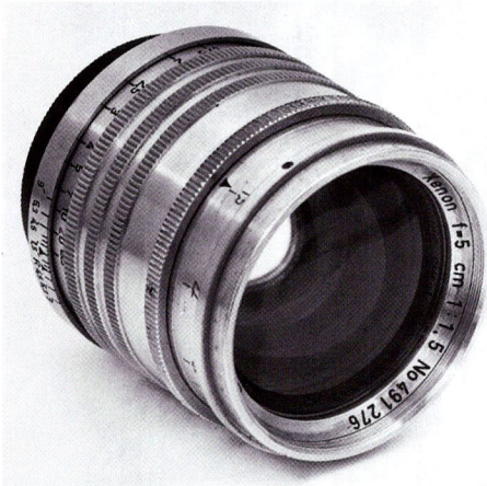
Xenon lens 491276 (circa 1941) with heavy front rim, X-ray application?
