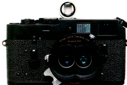
Leica M4 KE-7A from 1972, equipped with (uncommon) 3.3cm f/3.5 Stemar stereoscopic lens of much earlier construction and corresponding auxiliary finder.
