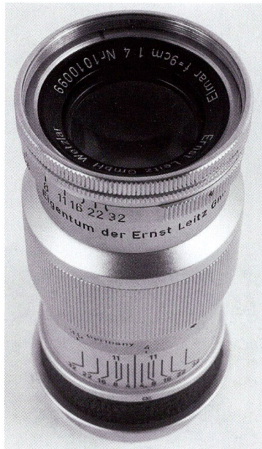
Unusual 9cm 1:4 Elmar lens 1010099 engraved "Eigentum der Ernst Leitz GmbH" meaning Leitz property. This specific lens is not entered in the shipping records associated with normal production lenses.
