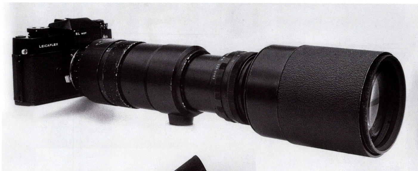
Massive 450cm 1:5.6 ELCAN "apochromat" lens prepared by Ernst Leitz Canada for the U.S. Navy. This is lens number three; probably less than ten were produced.
