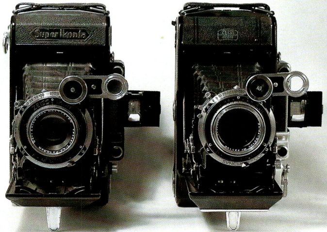
Super Ikonta 530/2 and 531/2 compared. The only difference is the double exposure safety lock near the shutter release button.
