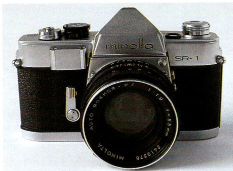
Minolta SR1 1414854, front view, with 55/1.8 Auto PF Rokkor no. 2419376. This lens maintains the yellow LV markings but has been updated with click marked diaphragm settings and the consequent removal of the release latch. The camera body also has an improved diaphragm mechanism that now opens following the shot independently of shutter cocking. The SR1 was also equipped with the 55/1.8. The exposure meter plate is contoured with two thin chrome strips, identical to the plate on the SR3.
