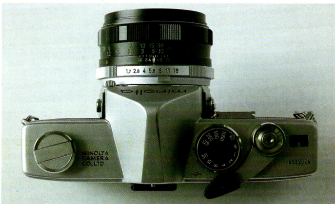
Minolta SR1s 4052024 seen from above. Note the self indexing tooth of the MC lens on the chrome aperture ring. It has no companion piece and is therefore not utilized because of the lack of a TTL meter. The advance lever has been modified once again. Covered in black plastic, it is identical in shape to the one on the SRT 101 of the same period. The SR1s offered 1/1000th and was the only SR1 model with this feature.
