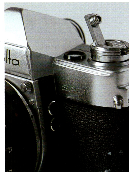
Detail of the FP and X synch terminals, frame counter, rewind lever and SR1 logo in green positioned on this side of the front to leave space for the exposure meter clip.
