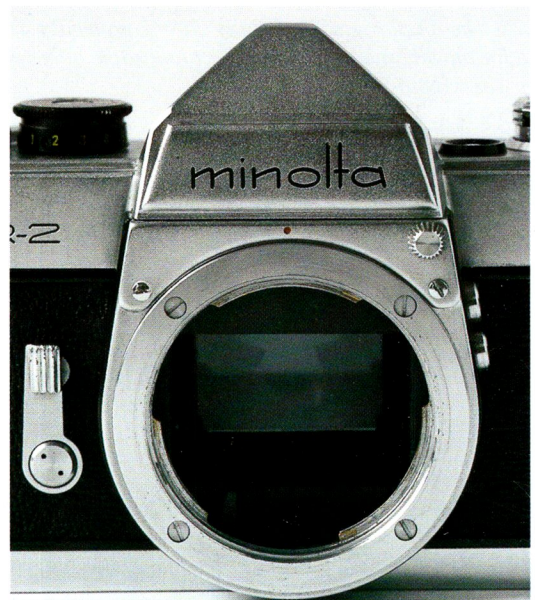
Detail of the lens changing catch and prism. Note the 3-prong bayonet that remained unchanged on all of this marque's non-autofocus models. The upper part of the self-timer lever hides the start knob of the self-timer itself. On the lower left, the lens changing catch with the automatic diaphragm release with a different shape and position than on later models to permit immediate opening. On the upper right, the traditional knurled lens release knob that remained unchanged right up to the SRT models of the 1980s. On the side, note the two X and FP synch terminals with standard coaxial connection.
