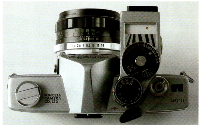
Minolta SR1s 4052024 seen from above with SR METER S. Basically identical to the SR METER V, it has a 1/1000th setting like the camera on which it was used. Note that neither the SR METER V or the SR METER S are marked with their names which only appear in the technical documentation. However, they are easily identifiable.
