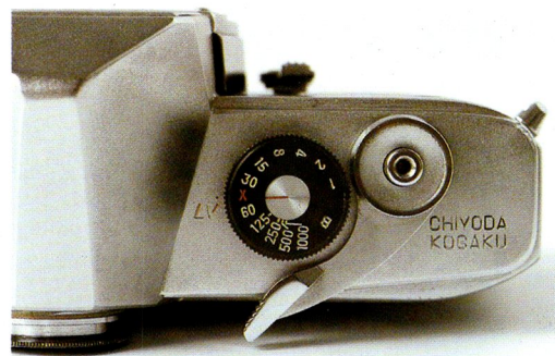
The SR2 advance lever and shutter speed dial. Note the irregularly-spaced times up to 1/1000th and the red 1/50th X sync positioned separately from the other timing sequence. The dial on the SR2 had to be lifted to be turned and it also turned freely from the bulb exposure to 1/1000th or 1 second. Also note the shutter release button housed in the fulcrum crown of the film advance lever, a position that would be maintained in all models up to the SRT and XM.
