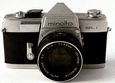
Minolta SR1 2055415, front view with lens. Note the tapering of the exposure meter plate prism; the unusual green color of the SR1 has been changed to the more traditional black. The uncommon 53mm focal length characterizes this amateur-market lens with speed setting limited to f/2. This focal length was not to be offered ever again.
