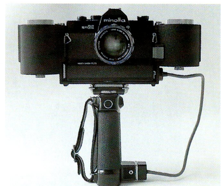
Minolta SRM 1001371, year 1970 with 250-shot back 111945 and 55/1.7 MC PF Rokkor 2752309 lens with which the SRM was equipped. The hand-grip attached to the back using a quick-shoe that contains the batteries that supply power to the SR motor, connected using the electrical cable visible on the right.
