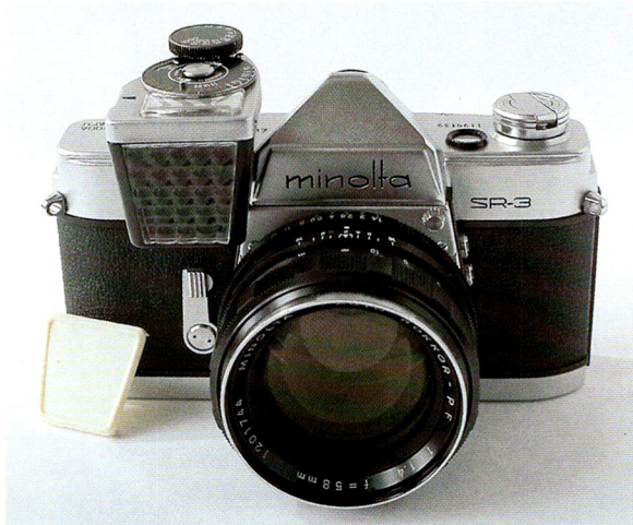
The SR3 with selenium exposure meter towering over the speed dial; below note the diffuser for reading incident light that could be inserted into the clip on the cell.
