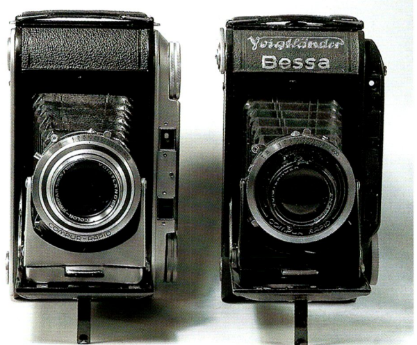
Pre-war Bessa E and Bessa II compared. There are a number of differences, including the coupled rangefinder viewfinder and different controls layout.
