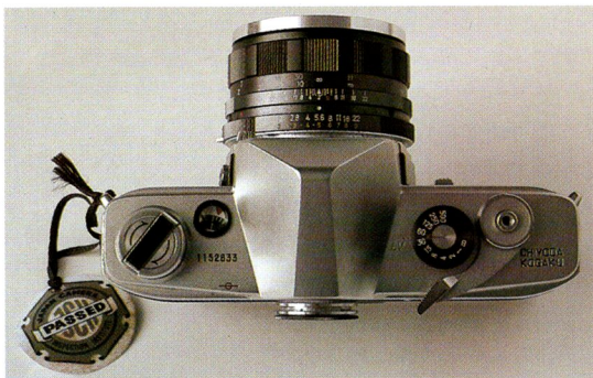
View of the SR1 from above. Note the speed ceiling of 1/500th and uniform spacing on the dial. This indicates its destination for amateur use as opposed to the SR2 and SR3 models that also included the prestigious 1/1000th. The lens kit was also more for amateurs with the modest 55/2 instead of the 55/1.8 and 58/1.4 of its more exalted brothers. Note the PASSED stamp.
