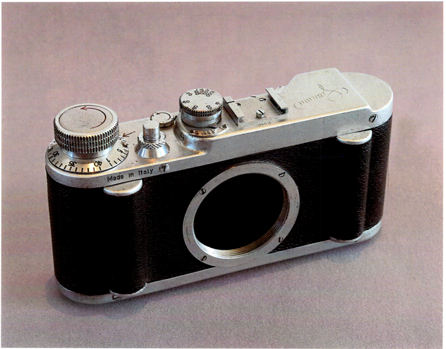
This, the last of the “out-of-the-ordinary” Gammas, bears the number 806, has long exposure times, screw mount and the same top plate as the R 803 but without a finder and rewind knob. It also has a film cutter the purpose of which is a total mystery to me!
