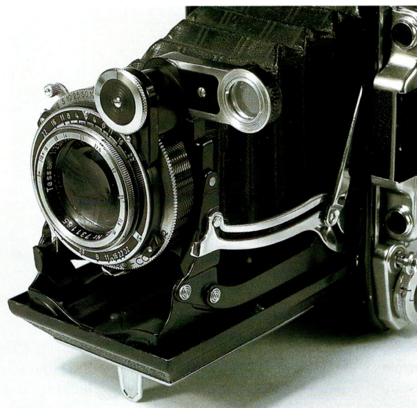
Detail of the Bessa II with Color Skopar lens and lens unit mounted on wheels for focusing.
