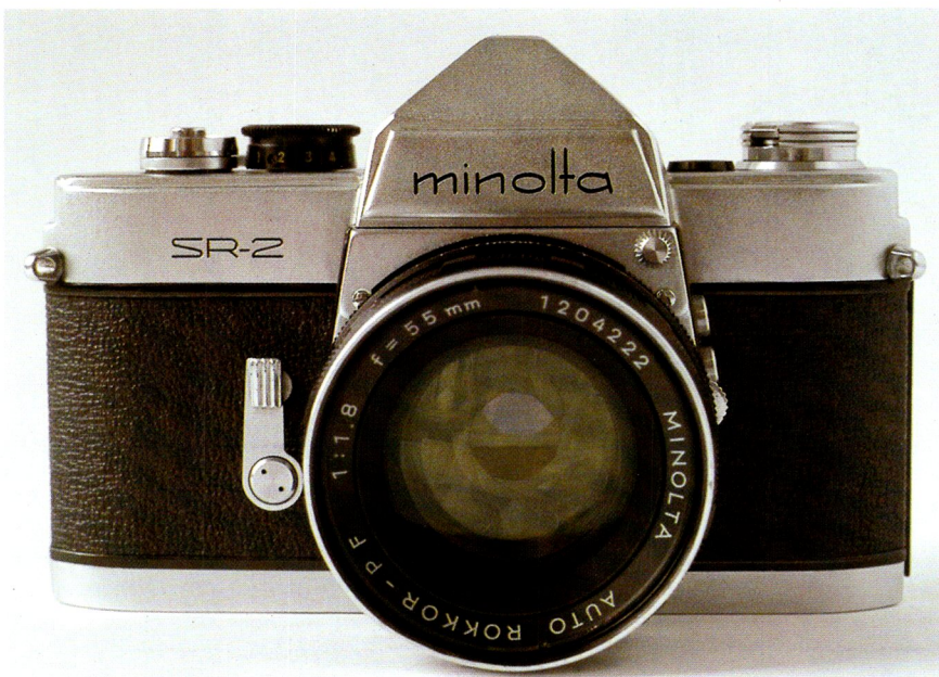
Minolta SR2 no. 1105836, year 1958. Front view with 55/1.8 Auto PF Rokkor no. 1204222. The diaphragm is partially closed, unusual for a mounted Minolta lens, but normal for the SR2 model in which the diaphragm only opened automatically when the shutter was wound-on.
