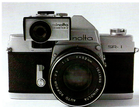
Minolta SR1 2055415, front view with SR Meter 2. Below the exposure meter body note the grooved black cover to the battery compartment; the CdS photocell is covered with a special calibrated blue filter for color correction.
