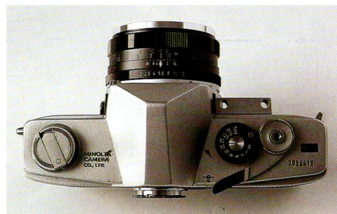
Note the different rewind button, the shifting of the frame counter from the left side to the extreme right and the changing of its shape from round to rectangular. The serial number position was also shifted along with that of the frame counter. The shiny end of the advance lever has changed shape, the exposure meter plate is squarer and its front is no longer contoured. The yellow LV markings are no longer to be found on either the body or lens.
