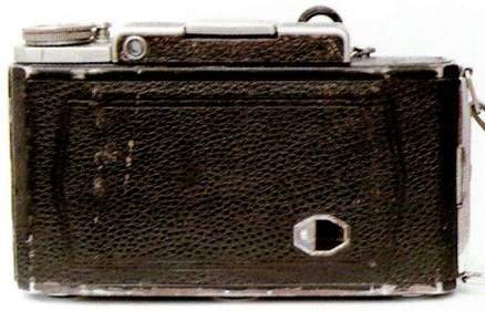
The back of the Moskva 2 with just the 6x9cm frame counter window.
