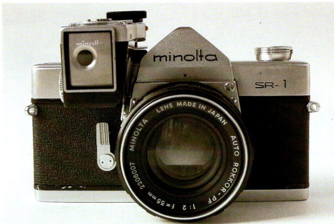
Minolta SR1V 2650946, front view, with SR METER V exposure meter. The hole in the center of the square on the front of the meter houses the CdS cell. Using the button on the side of the exposure meter, a drilled disk can be removed to select the more sensitive scale.
