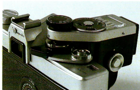
Minolta SR1s 4052024, detail of the body/exposure meter coupling mechanism. The prominent meter disk is hooked onto the tab on the shutter speed button. Note the button on the side of the meter. When pressed, it sets maximum film speed. When the crown is turned, it turns it on or selects the battery level check.
