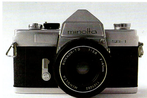
Minolta SR1 2418495, year 1964, model 5d with 45/2.8 TD Rokkor 1101062. Note the different shape of the self-timer lever that is identical to that later adopted on all SRT models; the same is also true of the rewind button. This is the last SR1 model before the switch to the V models and their totally revolutionized shape. Even if not indicated on the front ring, the 45/2.8 lens is automatic as on all previous models. The uncommon focal length and limited speed betray a Tessar-type lens scheme and the desire to create a unique piece. Its dimensions are quite limited, just 17mm wide and weighing only 130 grams. This lens, aimed at the amateur photography market, was not particularly successful and only a limited number (perhaps five thousand) were made, making it fairly rare.
