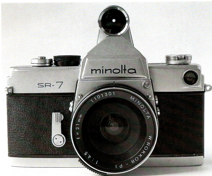
Minolta SR7 2122257, equipped with 21/4.5 W PI Rokkor 1101301 lens and its corresponding clip-on finder. This non retrofocus was set deep into the camera body and, at the time, could only be used by the SR7 with its manual mirror lock up mechanism.
