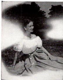
NEGATIVE ROLL LIGHT-STRUCK IN LOADING Note white streaks across picture. Do not break Scotch-Tape seal.
