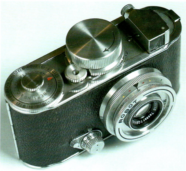
Robot I camera dated 1935, 24x24cm square format, the first successful spring-driven camera.
