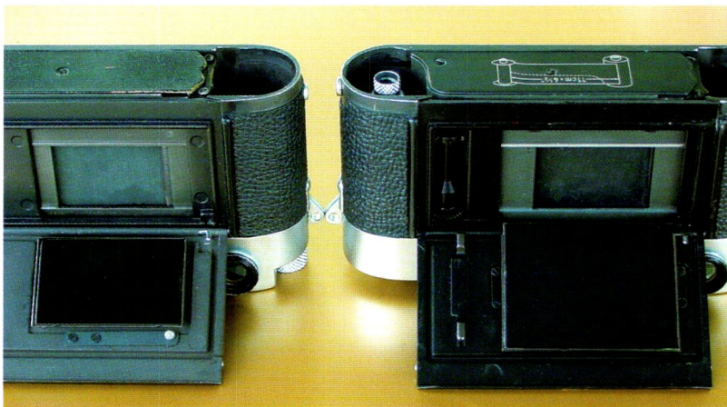
The interior of this M 005 is totally different than that of the M3, including its metallic structure. The plate that shields the moving parts on the bottom does not have the drawings that give instructions on how to load the film ...
