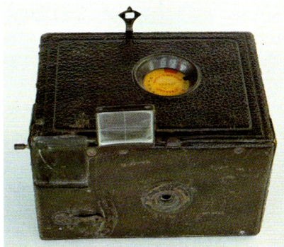
Le Pascal, probably the first spring-driven film advance camera.
