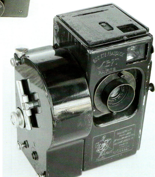
French Sept camera, derived from the Italian Autocinephot. The camera is equipped with a larger spring as can be seen from the box with the spring at the left.
