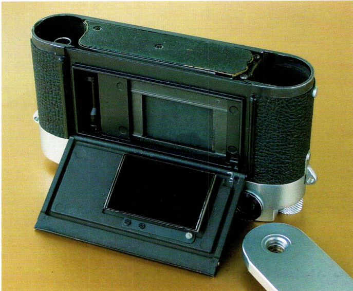
The interior of this M 005 is totally different than that of the M3, including its metallic structure. The plate that shields the moving parts on the bottom does not have the drawings that give instructions on how to load the film ...
