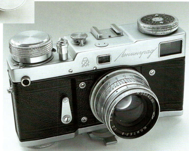
The GOMZ Leningrad with rangefinder, focal plane shutter and interchangeable lenses; produced from the mid-1950s to the end of the 1960s.
