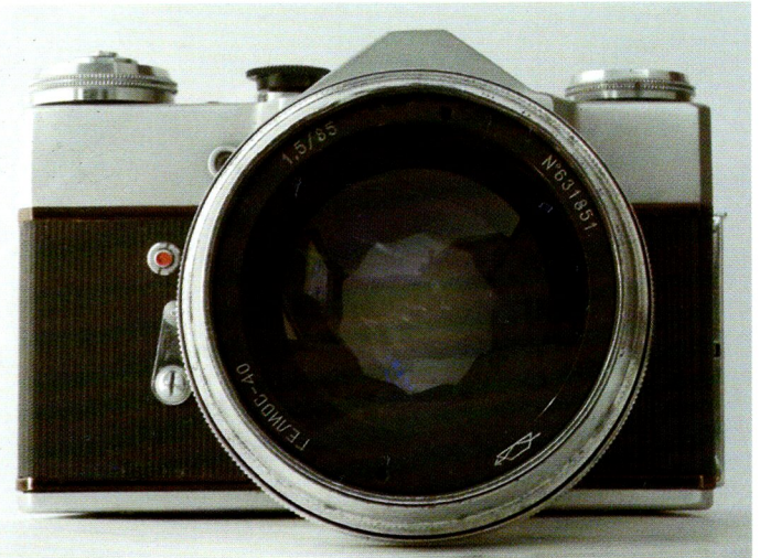
85mm f/1.5 Helios 40 mounted on a Zenit B reflex with 42x1 screw mount
