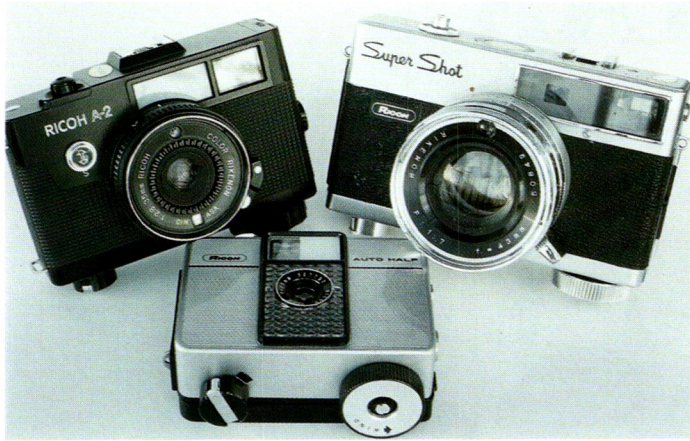
Three Ricoh spring-driven cameras, the 35mm Super Shot and A2 and the half-frame Auto Half.
