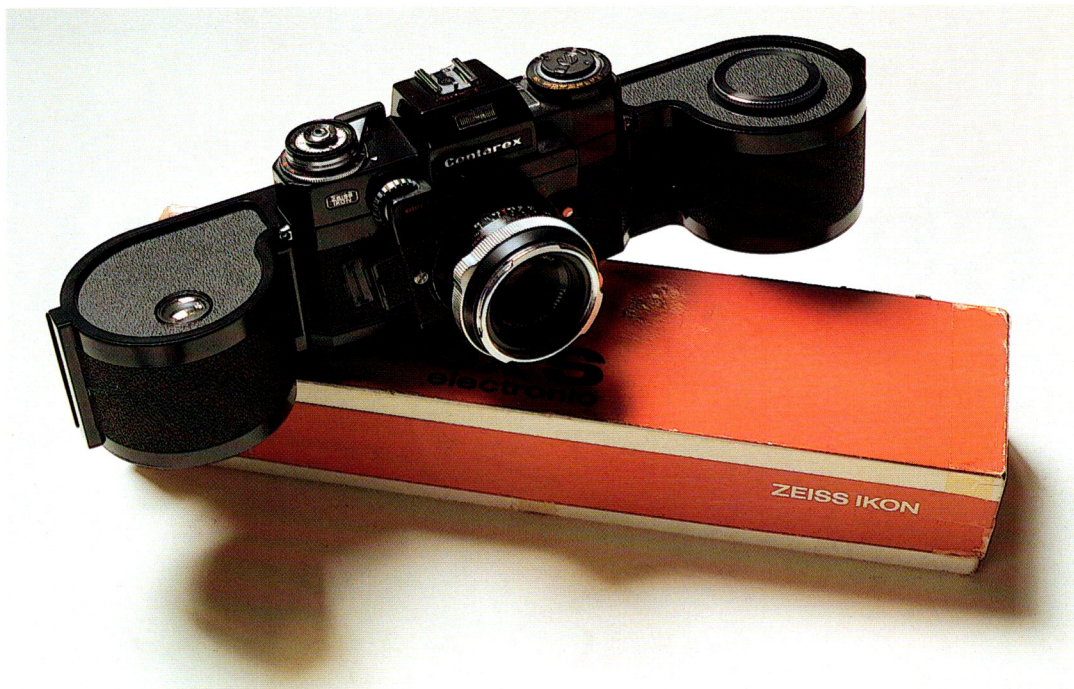
Back applied to the Contarex SE with frame counter window on upper surface
