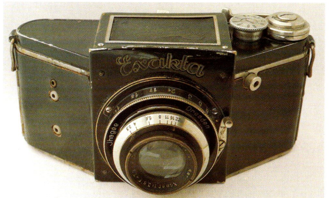
Exakta A, fourth type, with advance lever and Vacublitz synch socket
