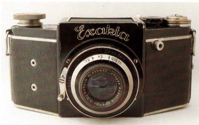
Exakta B, second type, with f/3.5 Exaktar lens, old mount, modified with advance lever and synch socket
