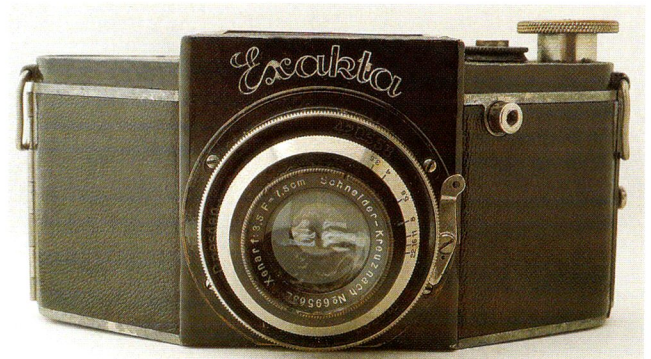
Exakta A, third type, with f/3.5 Xenar lens. New mount, release on left, wind knob and without synch socket
