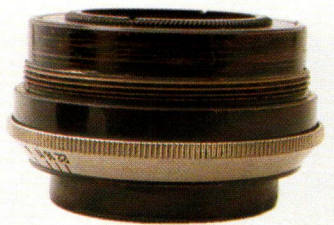
Lens with new mount 39.5 x 0.75
