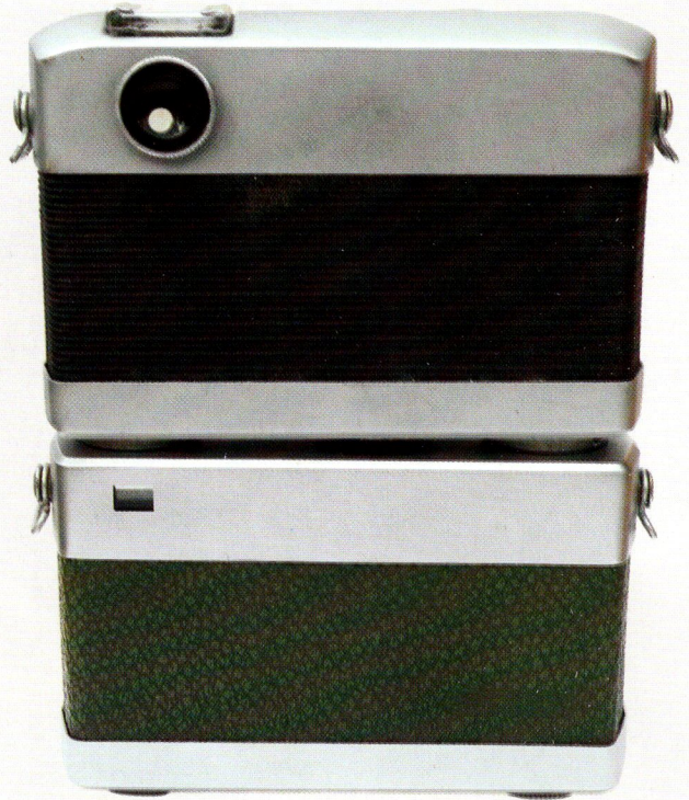
Werra I and Werra IE backs compared
