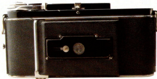
Exakta Junior with modified back for flat film
