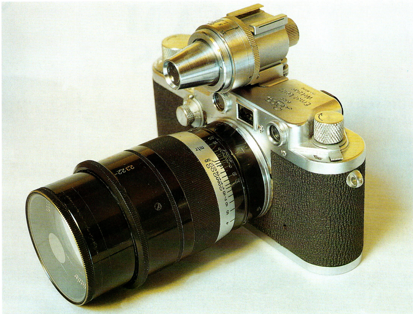
Thambar with filter inserted on Leica IIIc equipped with VIDOM multi-focal finder
