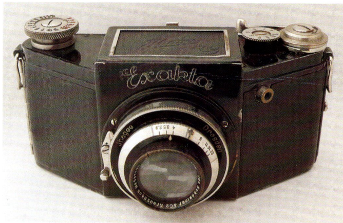
Exakta B, third type, with f/2.9 Xenar lens but with release lever on right
