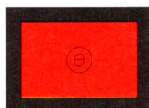
Metering field for large field integral metering as it appears in the viewfinder. To the right is a diagram of the lightpath with large field integral metering.
