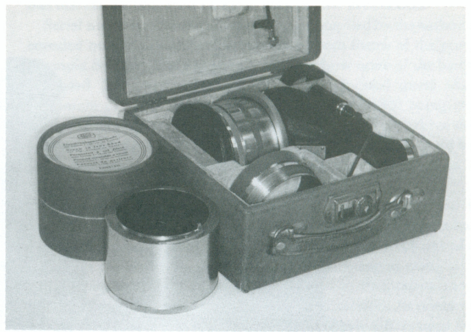
Prewar Flektoskop with extension tube in case. Sunshade and its container are to the left of the case.
