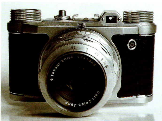
Altix V, 1956, 24x36mm format with 50mm f/2.8 Tessar interchangeable lens - front
