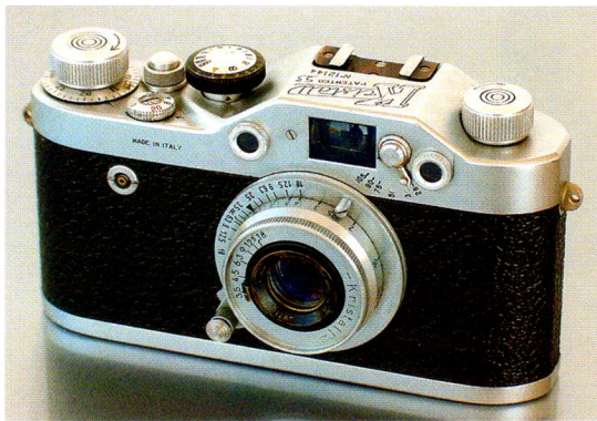
The Italian made Kristall camera series (in various models, 1954 -1955) often offered innovations on a technical scale. Models 2a, 2s and 3s were built in stainless steel and the Kristall 53, seen here, had a system of diaphragm adjustable viewfinders ranging from 28 to 105mm (1953, before the Leica M3). The 50mm f/3.5 Kristall lens is fully Leica compatible.
