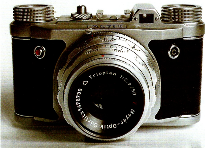
Altix V, 1954, 24x36mm format with 50mm f/2.9 Trioplan interchangeable lens and 1/250s Tempor shutter with red self-timer button on front - front
