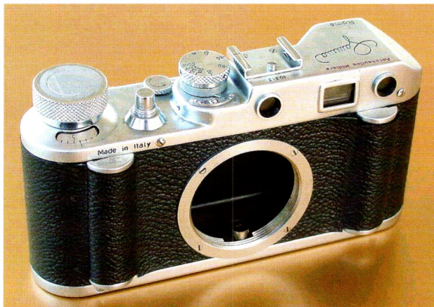
Despite the different position of the rangefinder lever which on the Gamma is placed on the lower part of the lens ring, it is 100% compatible with the Leica, including rangefinder.
