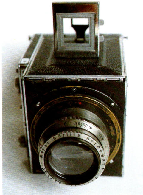
Primarflex front with frame finder open
