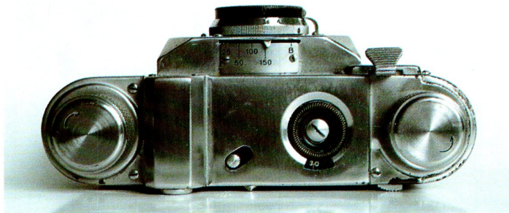
Altix I, 1939, 24x24mm format with 35mm f/3.5 Laack Pololyt - top plate
