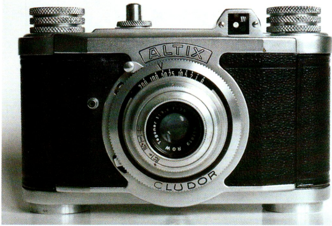
Altix II, 1949, 24x24mm format with 35mm f/3.5 ROW Tegonar interchangeable screw mount lens - front with name in block letters
