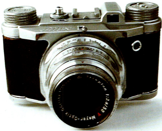
Altix V, 1956 (export model), 24x36mm format with 1/300s Prontor SVS shutter with linear shutter speed scale and 50mm f/2.9 Trioplan interchangeable lens - front
