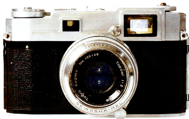
Topcon 35L with range finder, Seikosha MX leaf shutter and 44mm f/2 Topcor lens, front detail.
