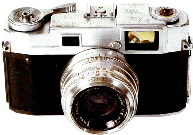
Topcon 35L with range finder, Seikosha MX leaf shutter and 44mm f/2 Topcor lens, front. The Topcon 35L (1957) had a selenium cell exposure meter that could be clipped on to the top plate and used the EV scale for rapid time-aperture selection.
