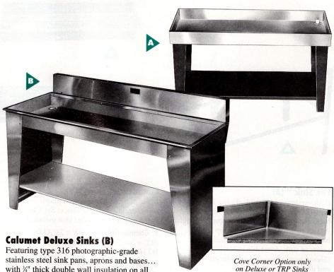
Featuring type 316 photographic-grade stainless steel sink pans, aprons and bases... with ½" thick double wall insulation on all four sides and bottom for better temperature control of processing. Bottom and sides are fully braced for maximum load strength. Includes 1½" stainless steel drain in rear right. Stand pipes optional.
