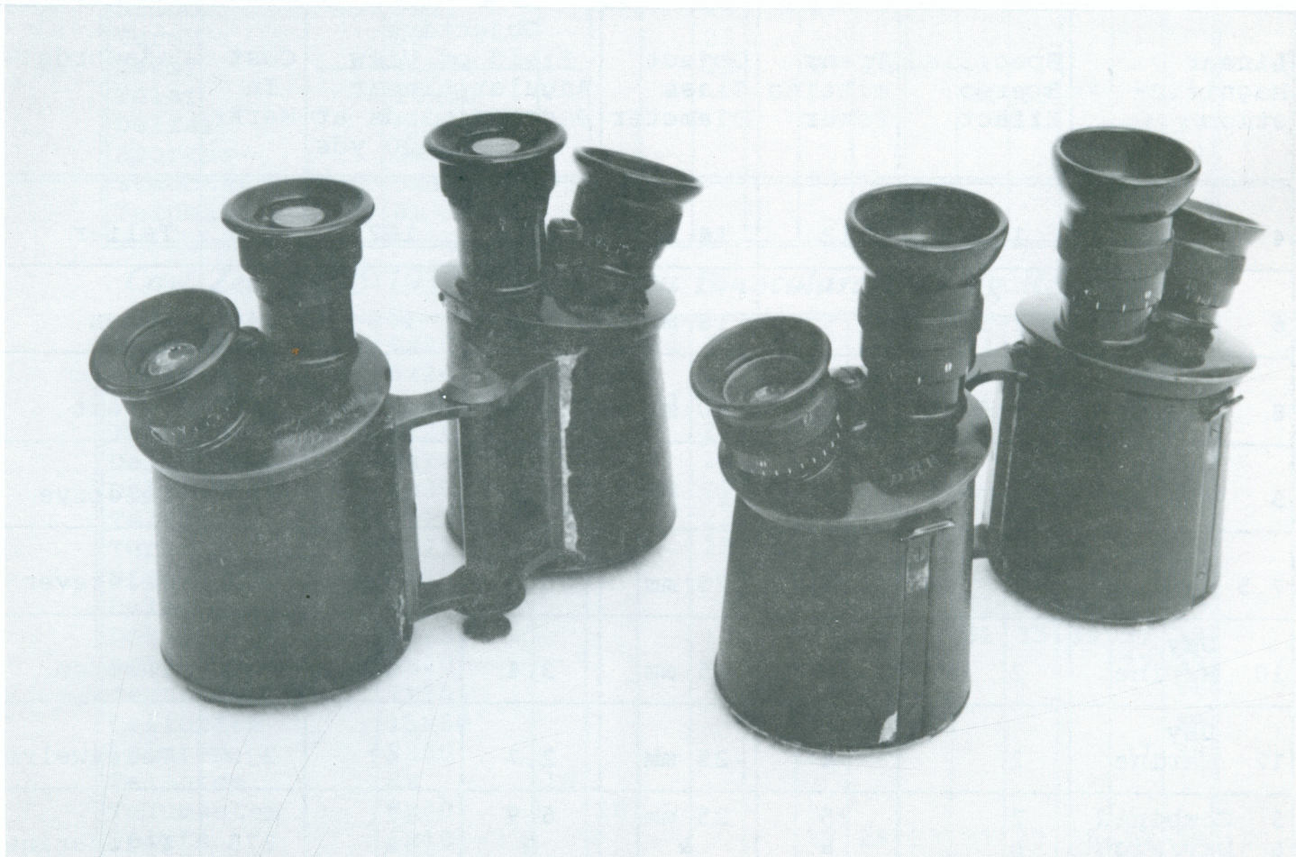
These revolving-eyepiece binoculars are examples of the rare Marineglas shown in the 1899 "Zeiss Prism Binoculars and Stereo Telescopes" catalog. One eyepiece gave 5-power magnification; the other, 10-power.
