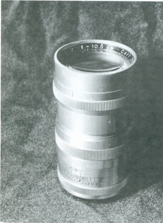
The mystery lens in its Leica screw mount. Next to knurled aperture ring can be seen f2 aperture marking.
