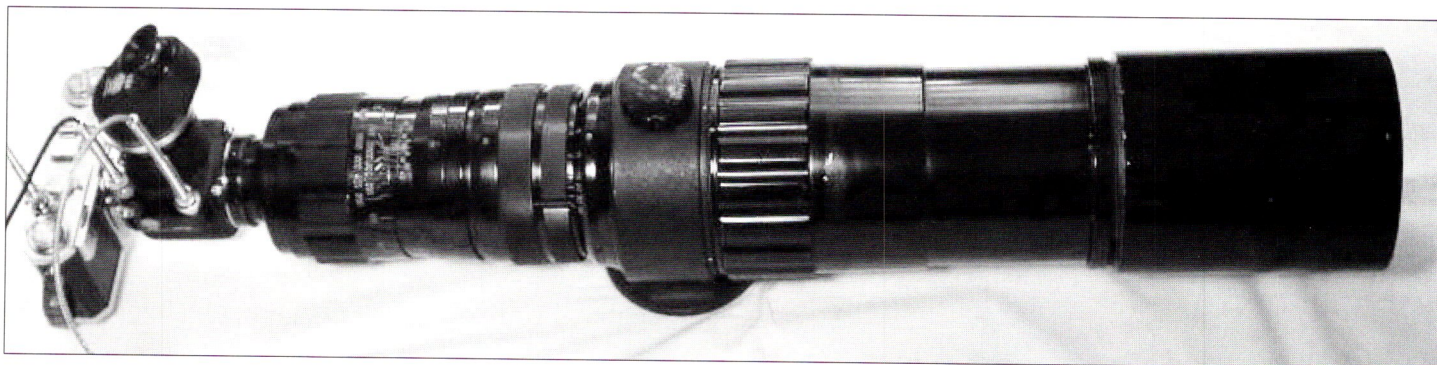
The 500mm f5 Nikkor-T mounted on the Type II reflex housing with a Nikon S2. One very long and heavy lens! At right is the drawing for the 500mm from Cooper & Abbott. It shows a lens calibrated in both feet and meters. This would be a very late vintage lens from possibly 1962 if they were actually made with both scales.
