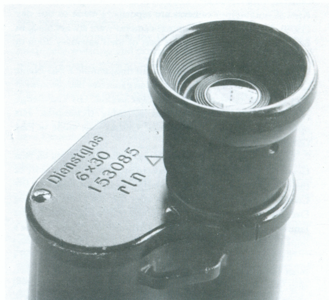
6x30 military monocular from Carl Zeiss Jena. Body is dark green-gray. All markings except the triangle are black enamel. The triangle is light blue, and its significance is unknown.
