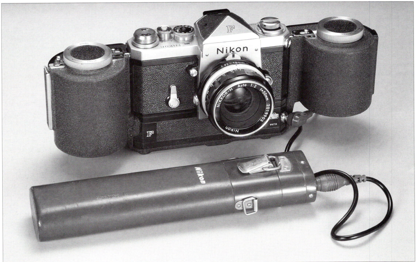
The F250 Motor Drive Bulk Back for the Nikon F in its original box with the early gray vinyl battery pack and matching gray cord. Even earlier examples can be found in a plain gray box with a dark blue bottom. Unlike all the bulk backs that followed it, the Nikon F version included the motor drive as well as the back. Later models used the 36 exposure motor while the back was a simple film chamber. Below is a slightly later model with the brown pack and black and gray cord. A well integrated and handsome design.
