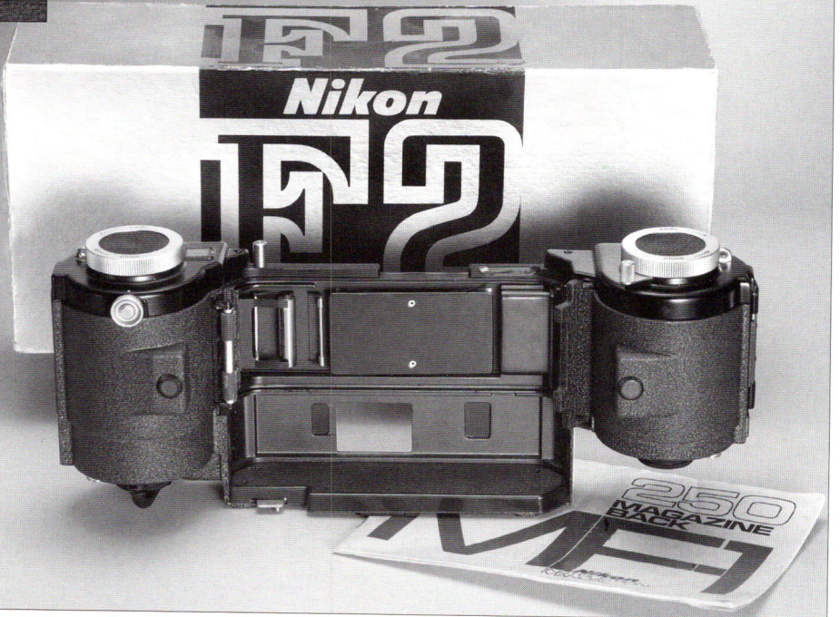
The 'Dummy' MF1/F2 mentioned in the text (upper right). Note 'Dummy' on the rear below the wind lever. The MF1 back is engraved 'No. A-6', a unique piece. Right..Brand new MF1 back with box and manual. Note that with the F2 you used your standard 36-shot motor and inserted it into the back housing. Below.. the MZ-1 cassettes for the F2 motor system. This design made loading the bulk backs quite easy.
