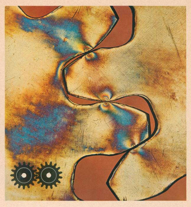
The two gears mesh. ZEISS Strain-Testing Devices reveal under polarized light the lines of principal stress. The centers of coloration show regions of maximum stress concentration. Thus ZEISS instruments have added new dimensions to materials research.
