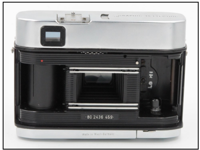
Figure 10: The serial number is just below the film plane.
