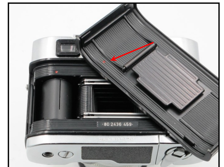
Figure 4: Film take-up drum in the Graphic 35 Electric housing the electric motor. The tiny red dots on the body and the back must be aligned when replacing the back.
