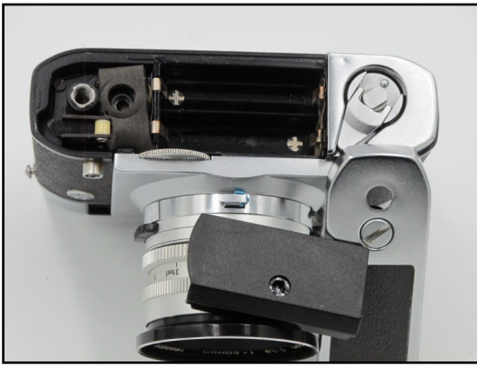
Figure 5: Battery compartment for the electric drive with insulating shield and baseplate cover.
