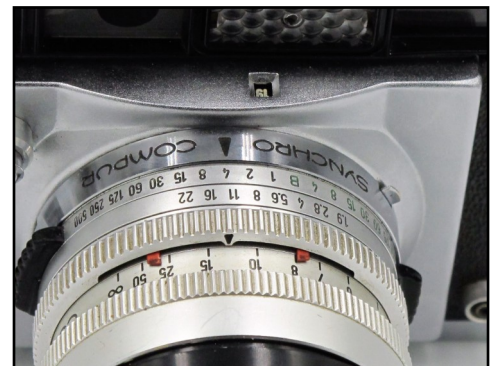
Figure 8: Depth of field indicator tabs integral with the shutter & mount mechanism. The frame counter window is just above the shutter.
