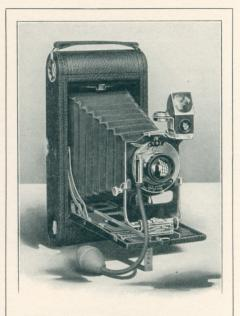
No. 3A Folding Pocket Kodak—For rectangular pictures  $3\frac{1}{4}$  x  $5\frac{1}{2}$  inches. Capacity, 10 exposures. Weight, 41 ounces. Lens, Rapid Rectilinear, speed f.8. Focal length,  $6\frac{1}{2}$  inches. Shutter, F. P. K. Automatic, with iris diaphragm stops, Nos. 4, 8, 16, 32, 64 and 128. Two tripod sockets. Rising and sliding front. Brilliant reversible finder with hood and spirit level. Automatic focusing lock.
