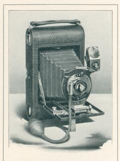
No. 3 Folding Pocket Kodak—For retangular pictures  $3\frac{1}{4} \times 4\frac{1}{4}$  inches. Capacity, 12 exposures without reloading. Size of Kodak,  $7\frac{1}{2} \times 4\frac{1}{2} \times 1\frac{1}{2}$  inches. Weight, 23 ounces. Lens, Rapid Rectilinear, speed f. 8. Focal length, 5 inches. Shutter F. P. K. Automatic, with iris diaphragm stops, Nos. 4, 8, 16, 32, 64 and 128. Two tripod sockets. Brilliant reversible finder with hood. Automatic focusing lock.
