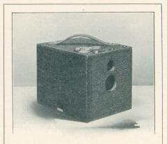
The No. 2 Bull's-Eye Kodak—For square pictures,  $3\frac{1}{2} \times 3\frac{1}{2}$  inches. Capacity, 12 exposures without reloading. Size of Kodak,  $5\frac{3}{4} \times 4\frac{5}{8} \times 4\frac{1}{2}$  inches. Weight, 22 ounces. Lens, Meniscus Achromatic, fixed focus,  $4\frac{1}{2}$  inches. Shutter, Eastman Rotary, with set of three stops. Brilliant finder and socket for tripod screw.
