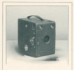
The No. 3B Quick-Focus Kodak—For rectangular pictures, 3½ x 5½ inches. Capacity, 10 exposures. Size of Kodak, 8½ x 6½ x 4½ inches. Weight, 2 pounds, 9 ounces. Lens, Meniscus Achromatic, focal length, 6½ inches. Shutter, Eastman Rotary, with set of three stops. Two brilliant finders. Two tripod sockets.
