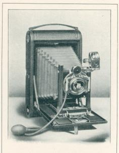
The No. 4A Folding Kodak—For rectangular pictures,  $\frac{1}{2}4 \times 6\frac{1}{2}$  inches. Capacity, 6 exposures. Size of Kodak,  $11 \times 6\frac{1}{2} \times 2\frac{5}{2}$  inches. Lens, Double Combination Rapid Rectilinear, speed f.8. Focal length,  $8\frac{1}{2}$  inches. Shutter, B. & L. Automatic, with iris diaphragm stops, Nos. 4, 8, 16, 32, 64 and 128. Rising and sliding front. Brilliant reversible finder with hood and spirit level. Two tripod sockets. Automatic focusing lock.
