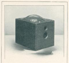
The No. 2 Flexo Kodak—For square pictures,  $3\frac{1}{2}$  x  $3\frac{1}{2}$  inches. Capacity, 12 exposures without reloading. Size of Kodak,  $5\frac{7}{6}$  x  $4\frac{5}{6}$  inches. Weight, 19 ounces. Lens, Single Achromatic, fixed  $4\frac{1}{2}$ -inch focus. Shutter, Eastman Rotary, with set of three stops. Finder.
